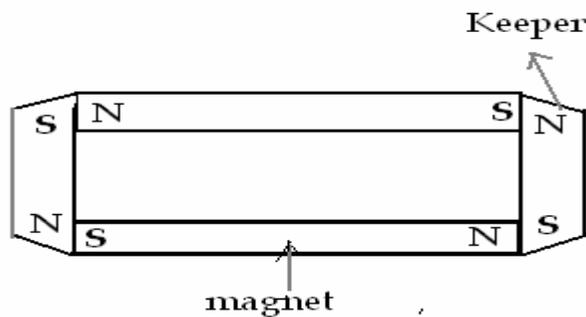
The keepers become induced magnets and their poles neutralize the poles of the bar magnets. The domains in both magnets and keepers form closed chains with no "free" poles.
