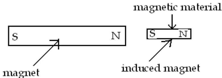
Induced magnetism can be used to form a “magnetic chain” as shown in the figure below. Each nail added to the chain magnetizes the next one by induction and attraction occurs between their adjacent unlike poles.
