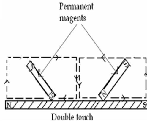
The methods of single and double touch are shown in figures a, b; Steel knitting needles, hair grips or pieces of clock spring can be magnetized. In single touch method, the steel is stroked from end to end about 20 times in the same direction by the same pole of a magnet.
